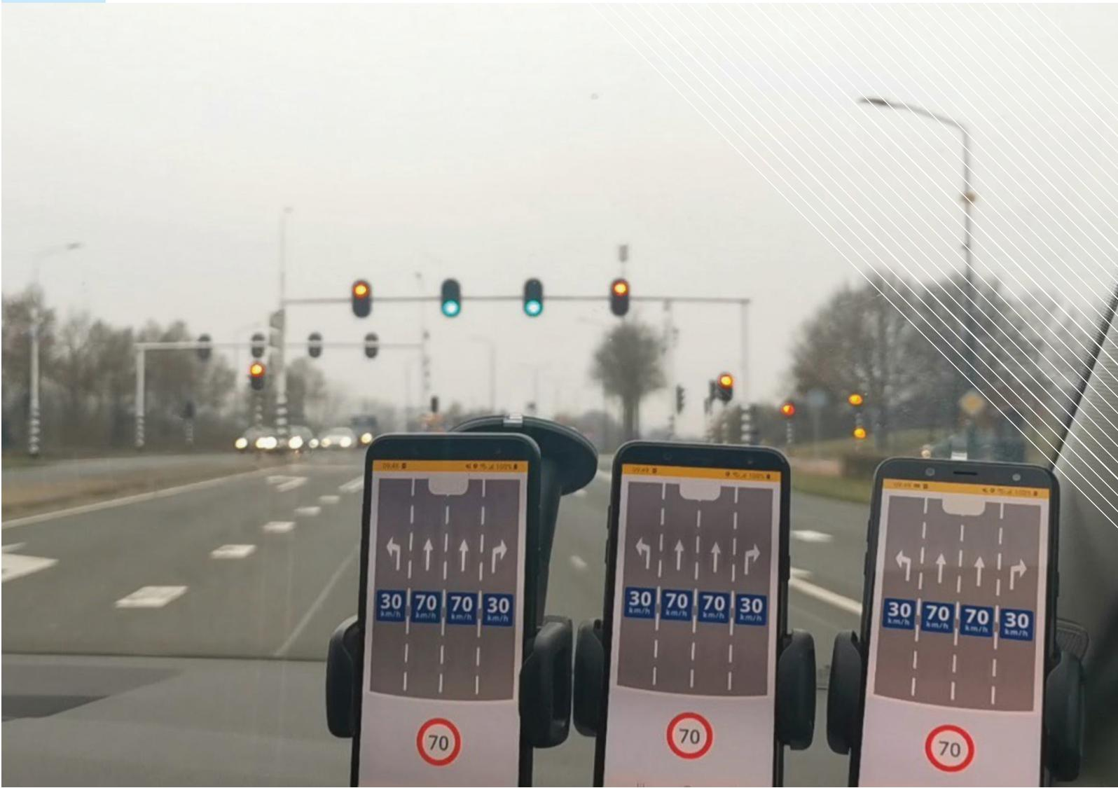
GLOSA stands for Green Light Optimal Speed Advisory. GLOSA supplies speed advice when passing through traffic lights. GLOSA's added value goes further than driver assistance alone. It is an important traffic management instrument which enhances quality of life and accessibility in urban environments.
