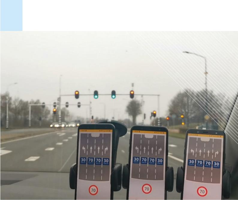
GLOSA stands for Green Light Optimal Speed Advisory. GLOSA supplies speed advice when passing through traffic lights. GLOSA's added value goes further than driver assistance alone. It is an important traffic management instrument which enhances quality of life and accessibility in urban environments.
